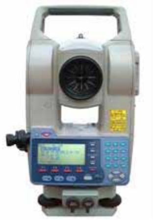
Figure 3. The developed light-wave survey camera with a built-in crack scale.
